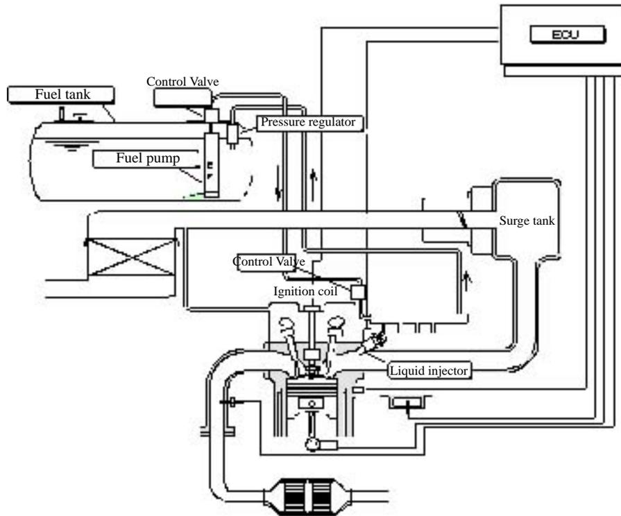
LPG Electronic Fuel Injection System (liquid injection)
