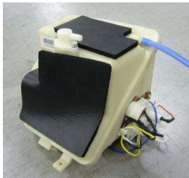
Figure 17. Example of insulation materials attached to the warm-water tank
