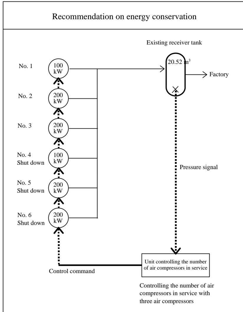
Figure II-6-9 Method of Controlling the Number of Air compressors
