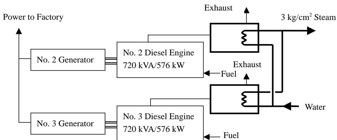
Figure I-6-1 Heat Recovery Method of the Exhaust Gas from Diesel Engines
