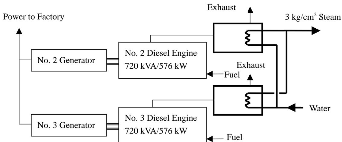
Figure I-6-1 Heat Recovery Method of the Exhaust Gas from Diesel Engines
