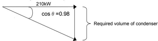
Required volume of condenser =  $210 \times \tan \theta = 210 \times 0.2 = 42\text{KVA}$
