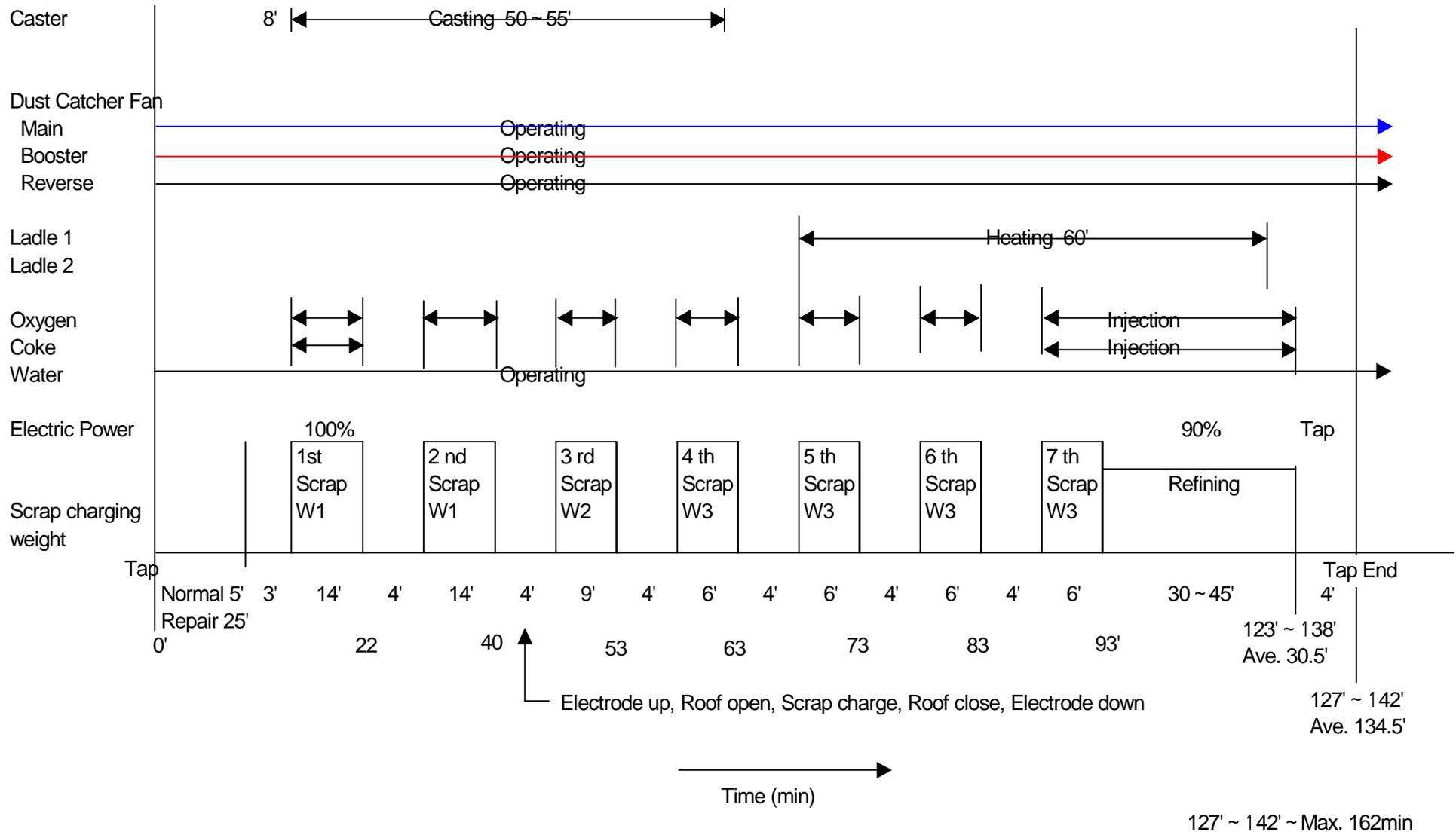
Figure II-6-1 EAF Operation Pattern in Company A
