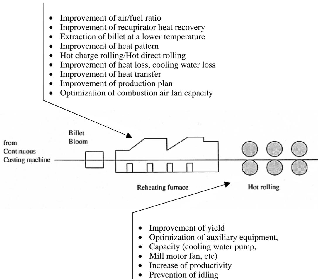
Figure II-7-8 Flow of Hot Rolling Process and Energy Conservation Measures
