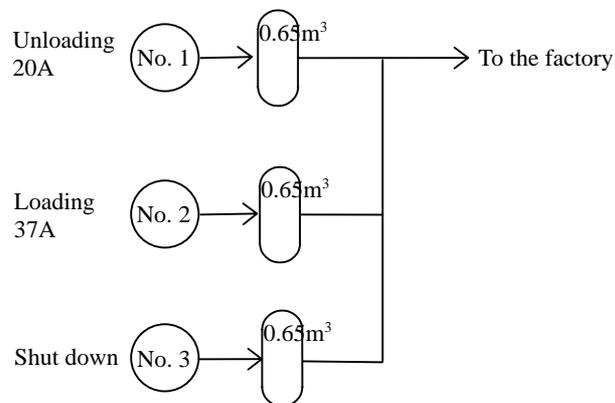
Figure II-4-1 Operating Method of Air Compressor
