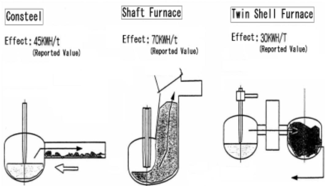
Figure II-7-6 Schematic Diagram of Scrap Preheating
