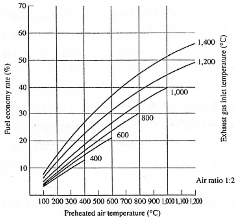
Figure II-7-12 Preheated Air Temperature Rise Effect
