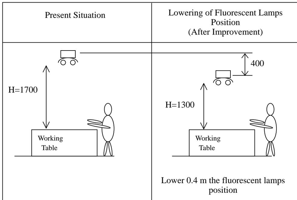
Figure I-6-6 Changing the Position of the Fluorescent Lamp on the Second Floor in the Old Factory
