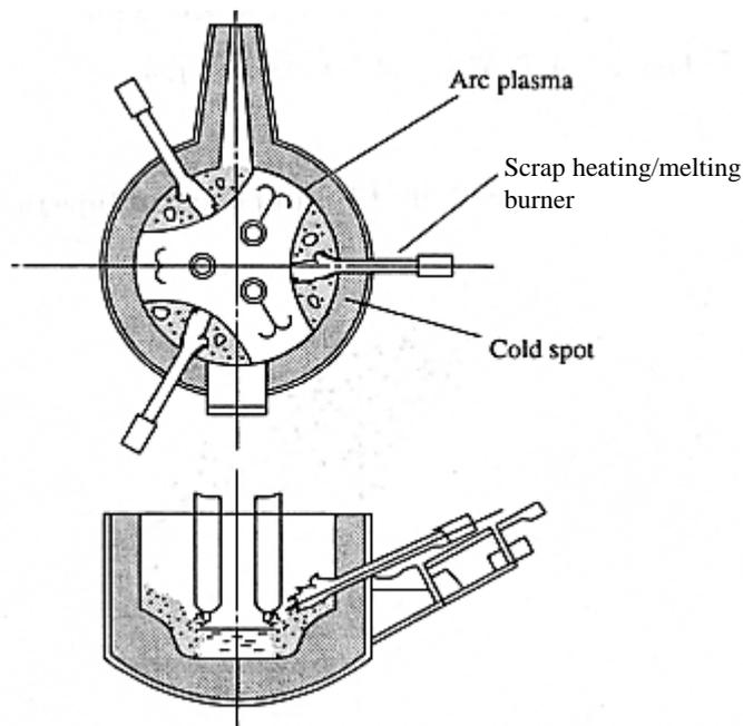
Figure II-7-4 Example of Providing the Scrap Heating/Melting Burner
