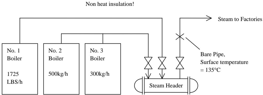
Figure I-6-3 Boiler Piping Schematic Diagram
