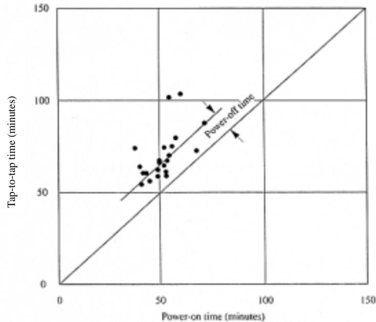
Figure II-7-7 Relationship Between the EAF's Tap-to-tap Time and Power off Time
