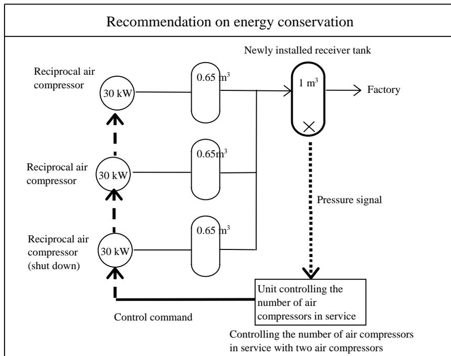
Figure II-6-5 Method of Controlling the Number of Air Compressors
