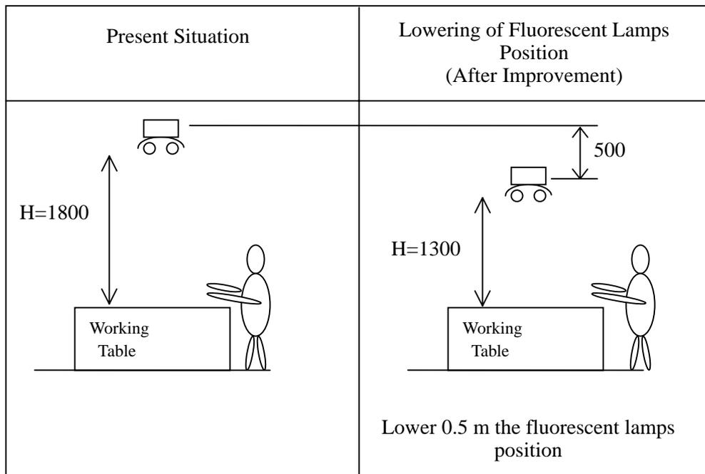
Figure I-6-5 Changing the Position of the Fluorescent Lamp on the Fourth Floor in the New Factory
