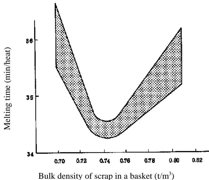
Figure II-6-2 Relationship Between the Scrap's Bulk Density and Melting Time
