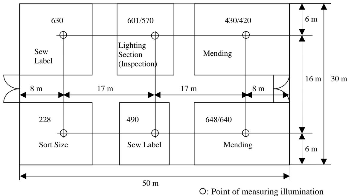
Figure I-5-3 Illumination through Ceiling Lighting ON/OFF in Shop A & B
