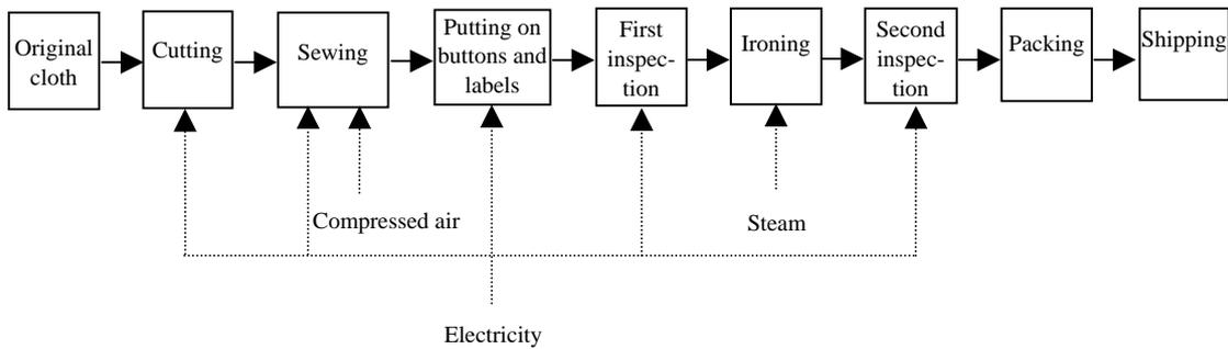
Figure I-7-1 Manufacturing Processes in the Garment Industry
