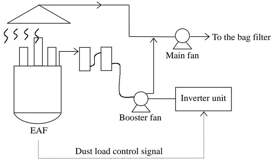
Figure II-6-4 Method of Controlling Revolutions of Dust collecting fan
