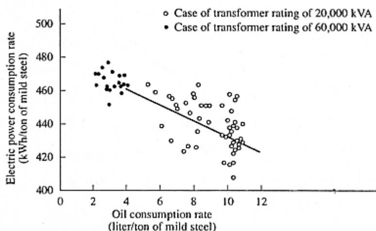
Figure II-7-3 Effect of Heavy Oil Burner on Reduction of Electric Power Consumption
