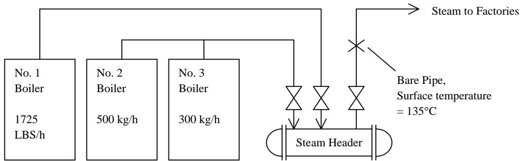
Figure I-5-4 Boiler Piping Schematic Diagram
