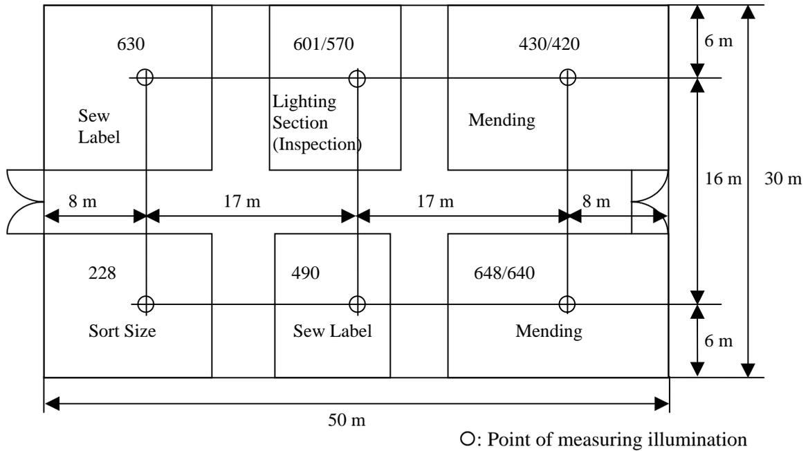
Figure I-5-3 Illumination through Ceiling Lighting ON/OFF in Shop A & B
