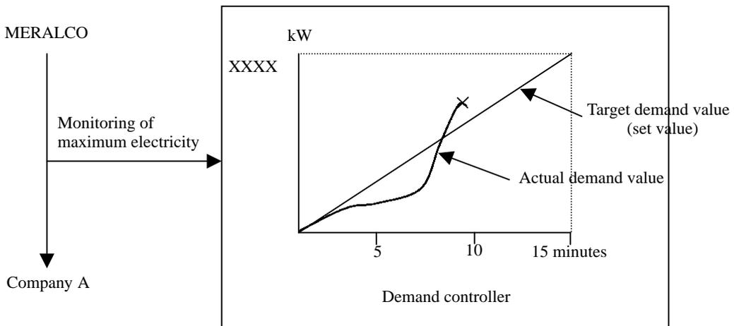
X: Since the target demand is likely to be exceeded, the load of the factory is partly limited or automatically shut down.
