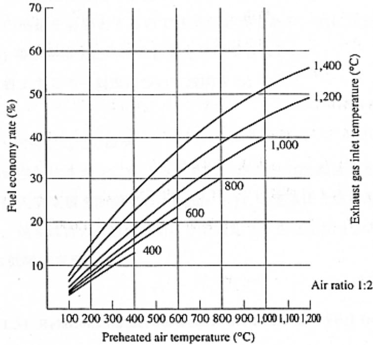
Figure II-7-12 Preheated Air Temperature Rise Effect
