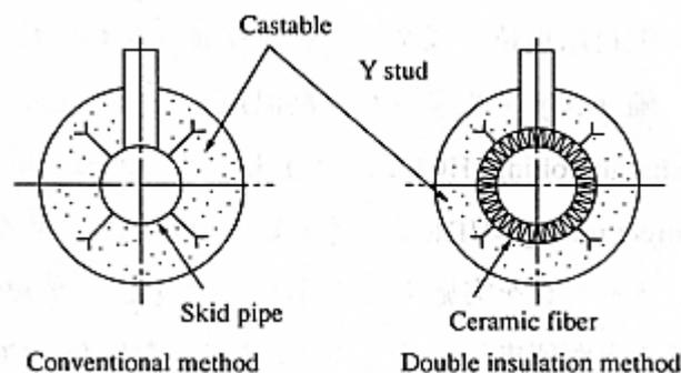
Figure II-7-10 Double Heat Insulation for Water-Cooling Skid Pipe
