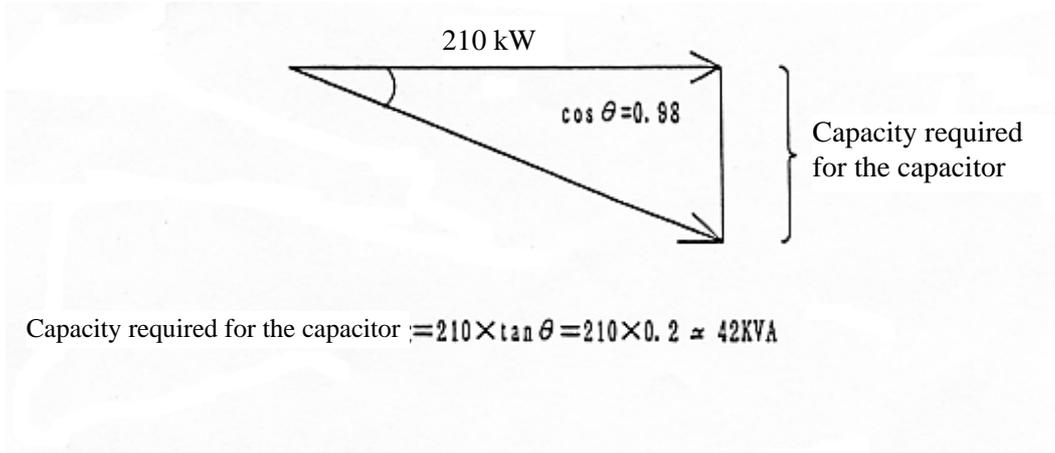
$$\text{Capacity required for the capacitor} = 210 \times \tan \theta = 210 \times 0.2 = 42 \text{ kVA}$$
