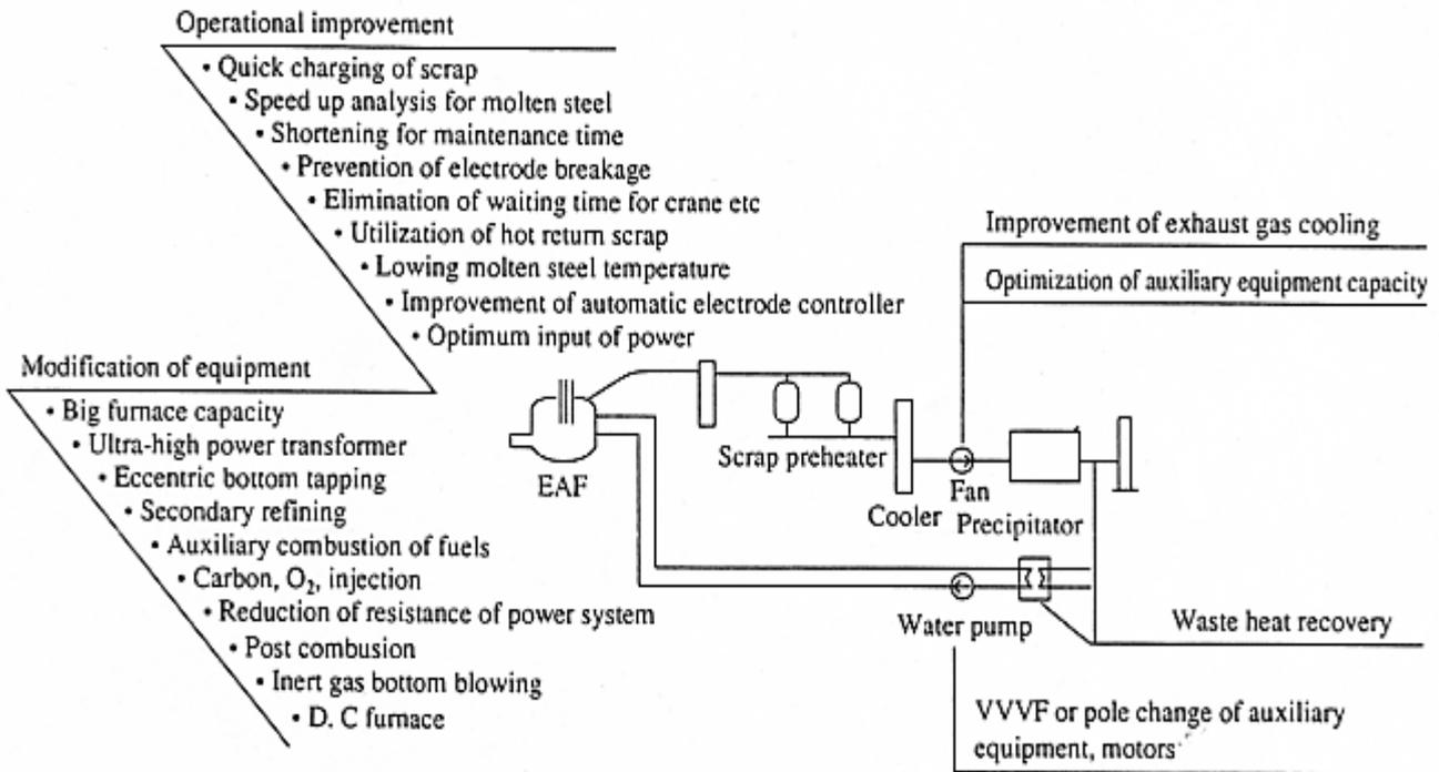
Figure II-7-2 Flow Chart of EAF Processes and Energy Conservation Measures
