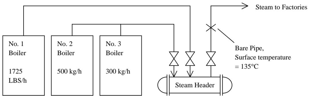
Figure I-5-4 Boiler Piping Schematic Diagram
