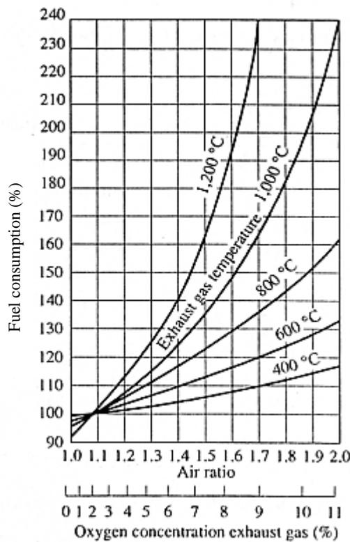
Figure II-7-9 Relationship Between Air Ratio and Fuel Consumption
