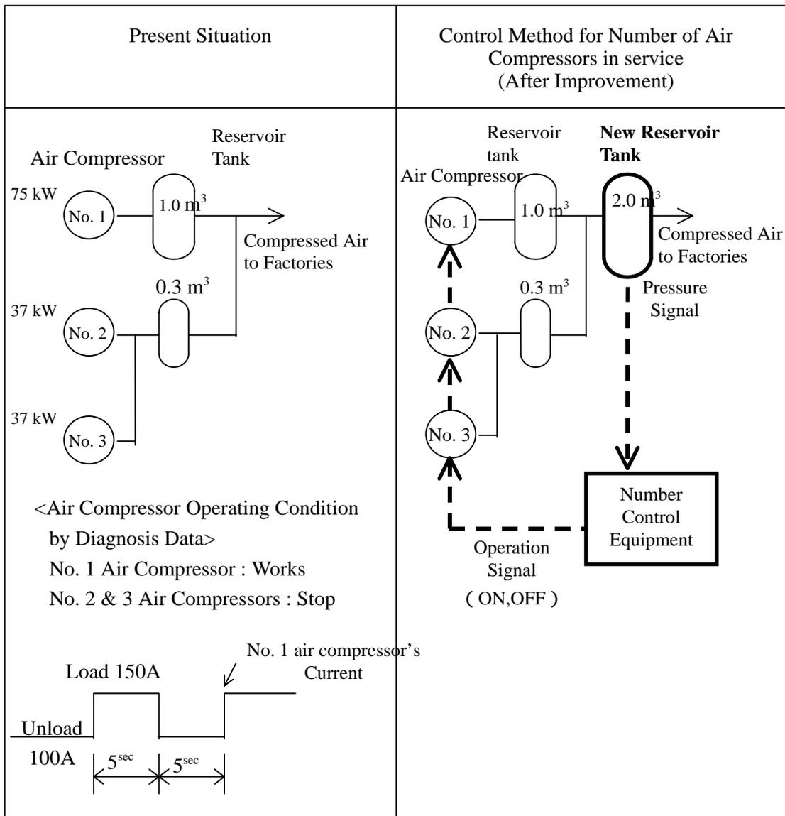
Figure I-6-4 Control Method for Numbers of Air Compressors in Service
