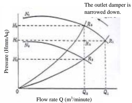
In contrast,  $N_1$  is reduced to  $N_2$  by controlling the number of revolutions, power reduces from the area of rectangle  $OH_1R_1Q_1$  to the area of  $OH_3R_2Q_2$ .
