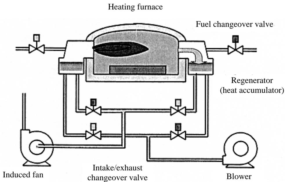
Figure II-6-6 Schematic Diagram of Heating Furnace Using Regenerative Burner
