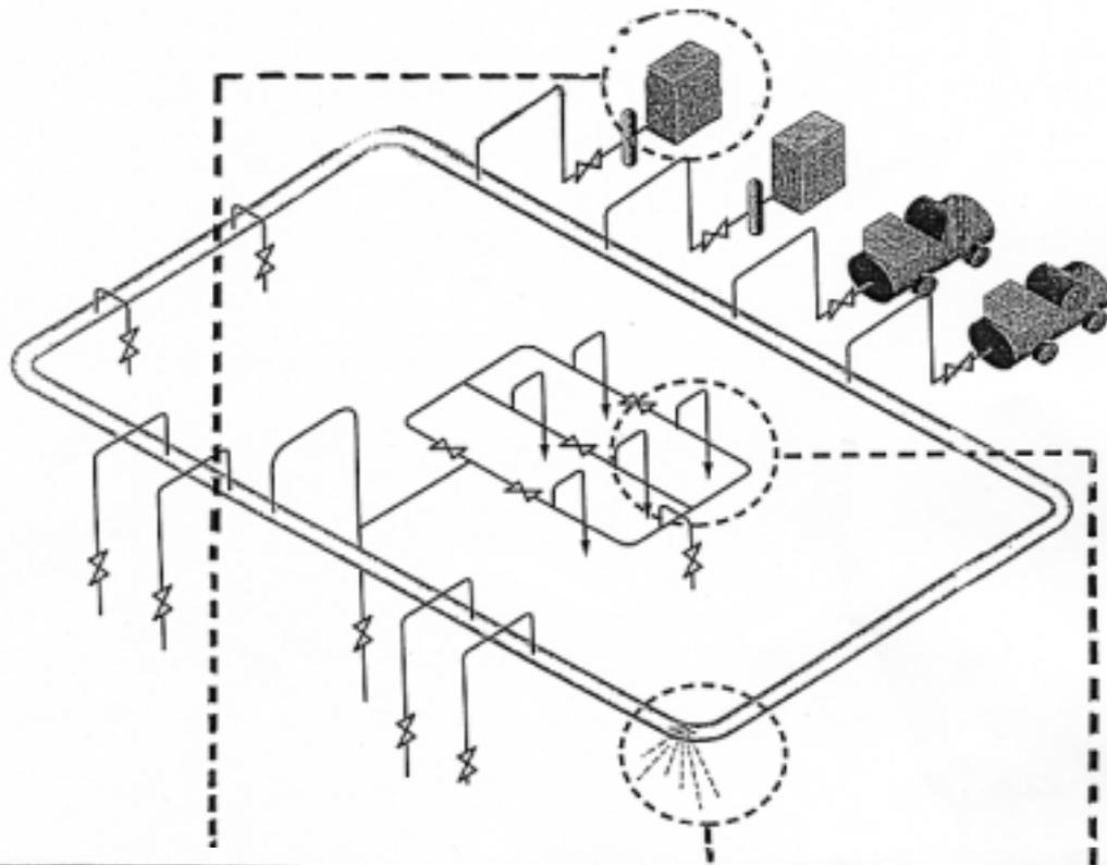
(1) Renewal to a new machine (high-efficiency air compressor)
