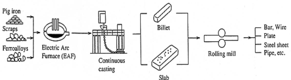
Figure II-7-1 Process Flow of Material and Product in a Factory with EAF
