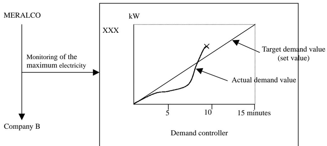
X: Since the target demand is likely to be exceeded, the hazard light issues an alarm at this point. With this alarm, the load is limited to the value that the production activities are not obstructed and the maximum electricity is suppressed below the targeted demand value.
