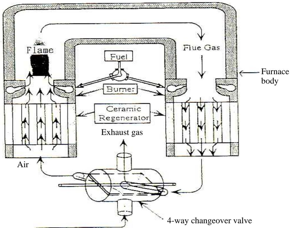
Figure II-7-11 Regenerative Burner System
