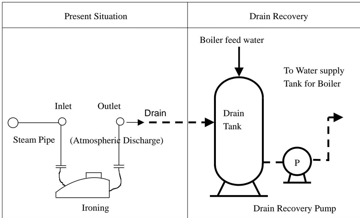
Figure I-6-2 Drain Recovery Method from the Ironing Process
