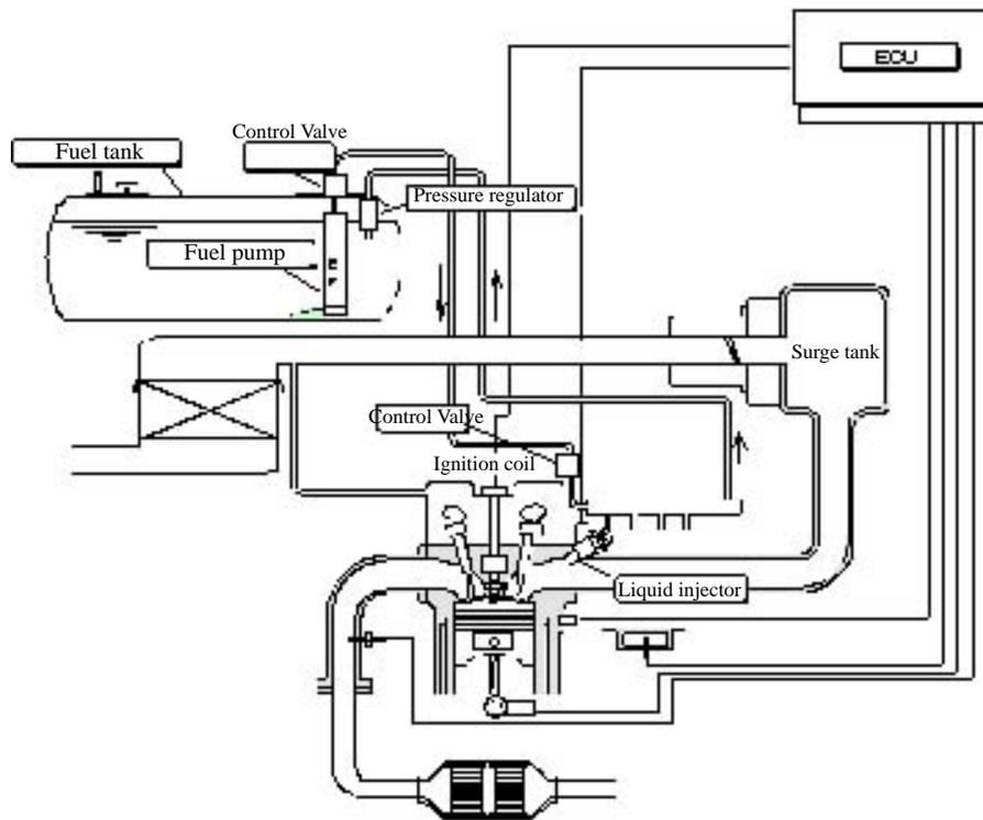
LPG Electronic Fuel Injection System (liquid injection)
