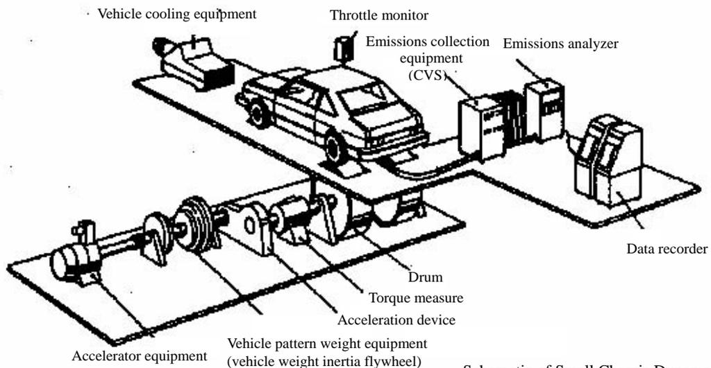
Schematic of Small Chassis Dynamometer
