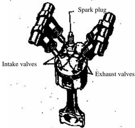
● Four valve combustion chamber
