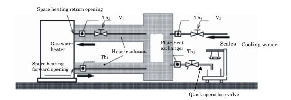
Figure 1: Heat Efficiency Test Device (Example)
