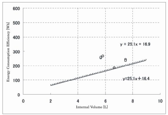
Figure 6: Internal Volume – Energy Consumption Efficiency (Grill Section) (Single-sided without water)
