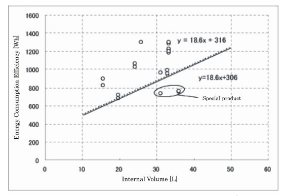
Figure 10: Internal Volume – Energy Consumption Efficiency (Oven Section) (Tabletop and Cabinet/stationary type)
