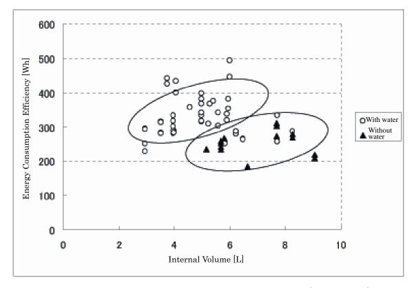
Figure 2: Internal Volume – Energy Consumption Efficiency (Grill Section)
