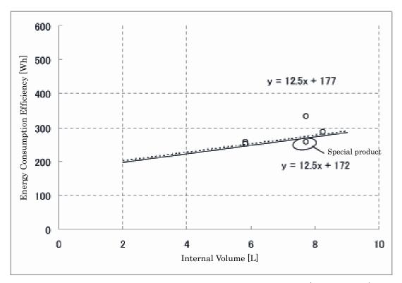
Figure 7: Internal Volume – Energy Consumption Efficiency (Grill Section) (Double-sided with water)
