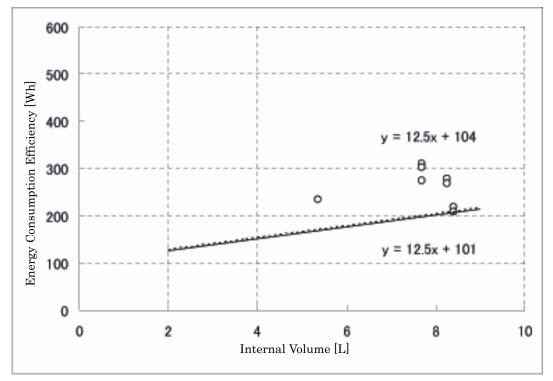
Figure 8: Internal Volume – Energy Consumption Efficiency (Grill Section) (Double-sided without water)
