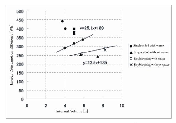
Figure 4: Internal Volume – Energy Consumption Efficiency (Grill Section)
