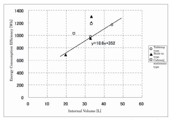
Figure 9: Internal Volume – Energy Consumption Efficiency (Oven Section)
