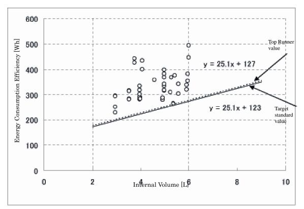
Figure 5: Internal Volume – Energy Consumption Efficiency (Grill Section) (Single-sided with water)
