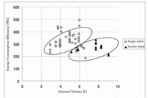
Figure 1: Internal Volume – Energy Consumption Efficiency (Grill Section)
