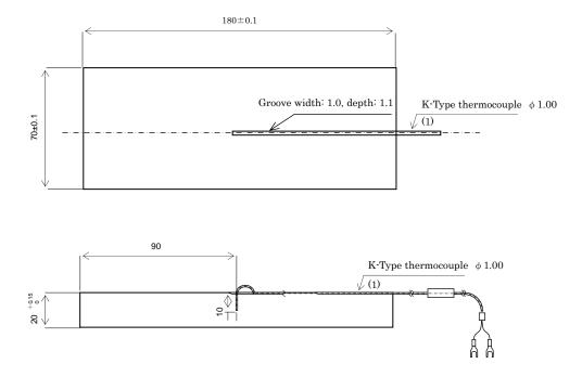
Figure 1: Thermocouple Installation
