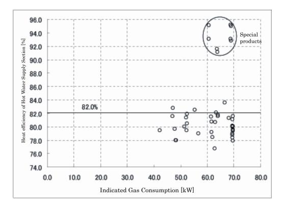
Figure 7: Heat Efficiency of Hot Water Supply Section in Category B
