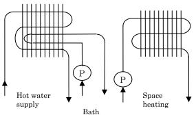
C. Two chambers with two flow channels
