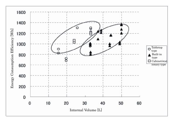
Figure 3: Internal Volume – Energy Consumption Efficiency (Oven Section)
