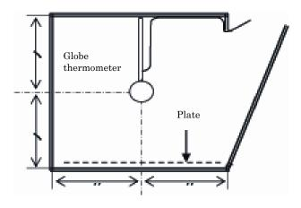
Figure 2: Globe Thermometer Installation
