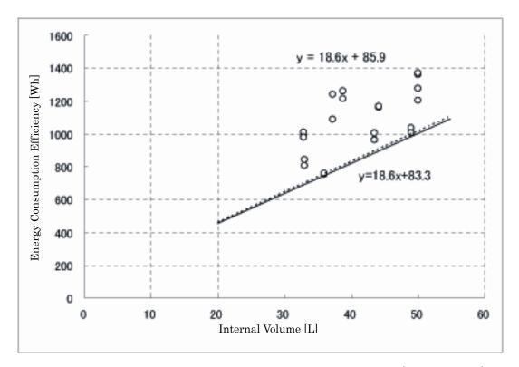
Figure 11: Internal Volume – Energy Consumption Efficiency (Oven Section) (Built-in Type)
