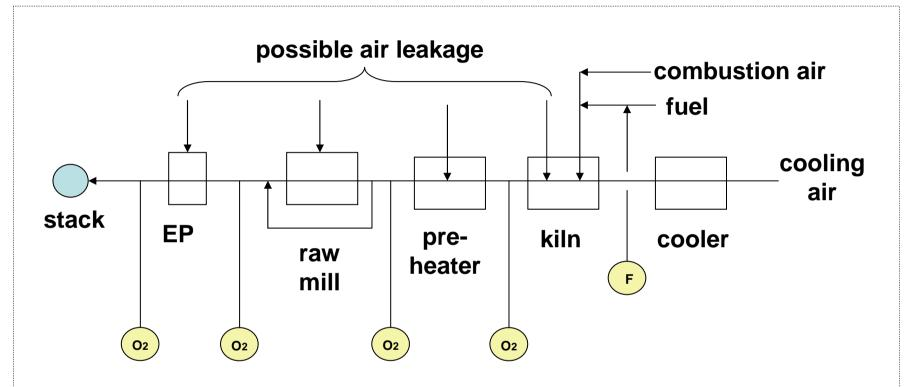
Air leakage may bring about an increase of both fuel consumption and fan power consumption.
