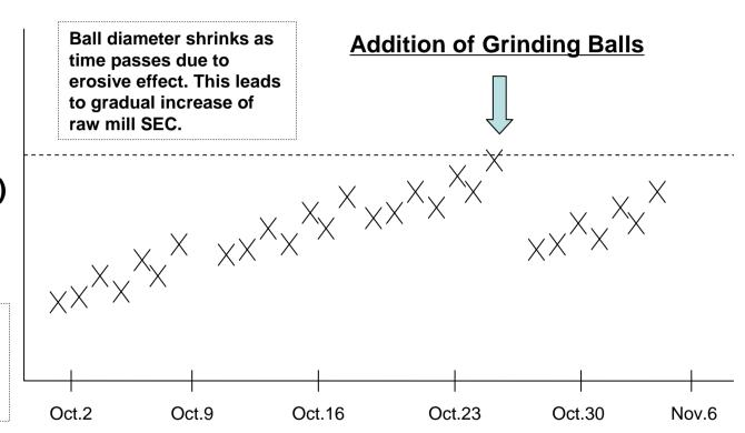
Monitor raw mill SEC daily and add grinding balls in right timing 10% energy saving expected
